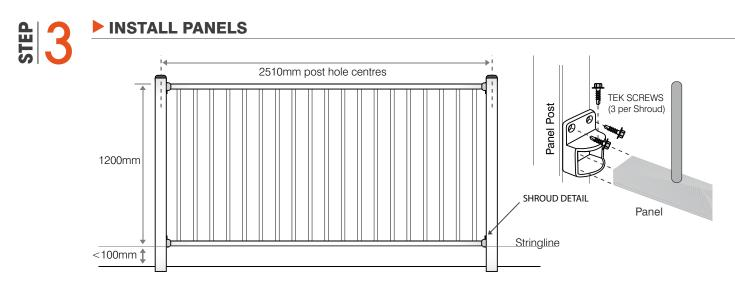
Using your string-line as a guide for the position of the bottom rail of the panel, fix the panels to the posts with the shrouds/brackets with self-tapping tek screws. If required, the panels can be attached to the shrouds at up to a 30° horizontal angle.
