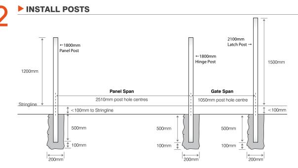
Measure the distance from the string-line to the top of the post, allowing 50-100mm under the 1200mm high panels. Then allow 10-20mm from the top of the panel to the top of the post.
